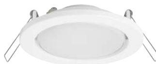
CHICO GX IP20/IP44 5W/828 110D WH LED 5W 300LM 2800K 15 000H BEAM ANGLE 110° Valkoinen | Vit | White
