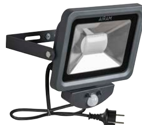
LED FLOODY PIR IP44 30W/840 2100LM LED 30W 2100LM 4000K 35 000H BEAM ANGLE 120° Antrasiitti | Antracit | Anthracite
