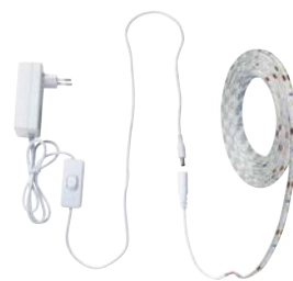
LED STRIP 12V 14,4W 3M LED 4,8W/M 240LM/M 3000K 15 000H Valkoinen | Vit | White
