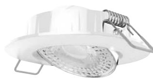
COSMO IP20 5,8W/830 DIM WH LED 5,8W 480LM 3000K 25 000H BEAM ANGLE 36° Valkoinen | Vit | White
