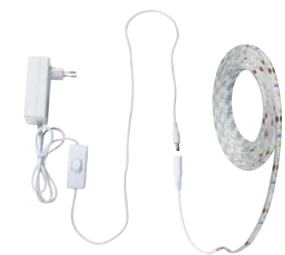
LED STRIP POWER 12V 21,6W 3M LED 7,2W/M 500LM/M 3000K 15 000H Valkoinen | Vit | White
